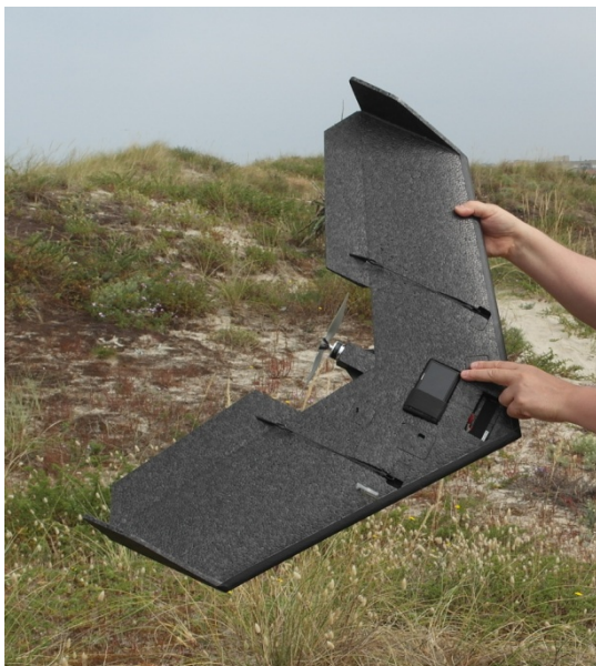
Figure 2. The swinglet CAM with the camera onboard (Photo by R.Henriques, 2014)
